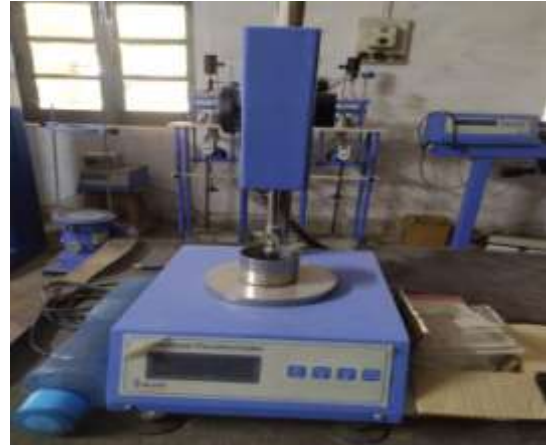
Figure 3. Cone penetrometer apparatus
